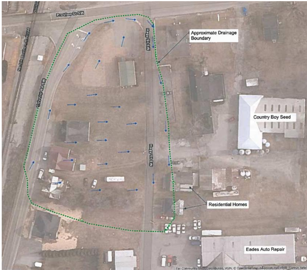
Figure 4. Preston Street Existing Drainage Pattern
