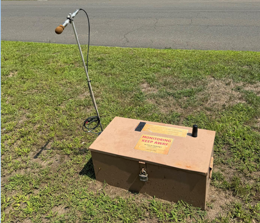
Vibration Monitoring Unit at OU4
